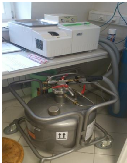
Slika 11. DSC instrument Mettler Toledo DSC 822°
