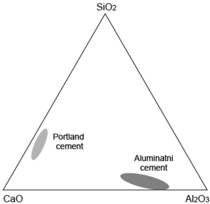
**Slika 1.** Sastav aluminatnog cementa u sustavu  $\text{CaO}-\text{SiO}_2-\text{Al}_2\text{O}_3$
