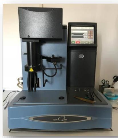
**Slika 21.** Termogravimetar, Q500, TA Instruments
