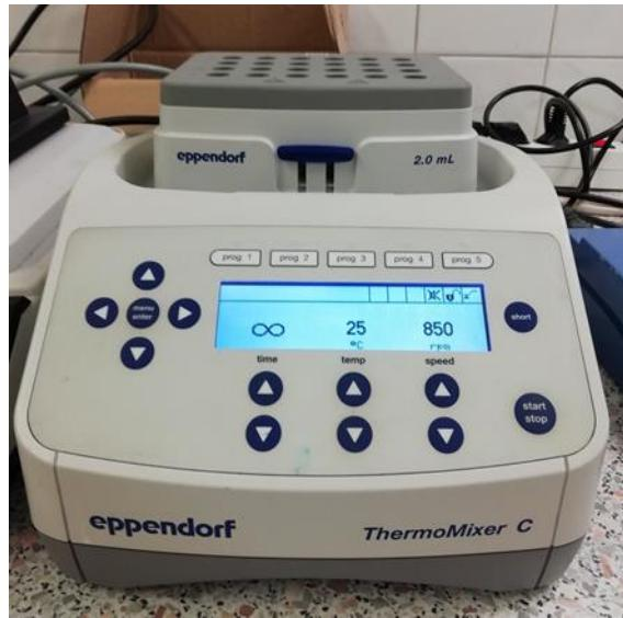
**Slika 10.** Termostatirana tresilica *Eppendorf ThermoMixer C*.
