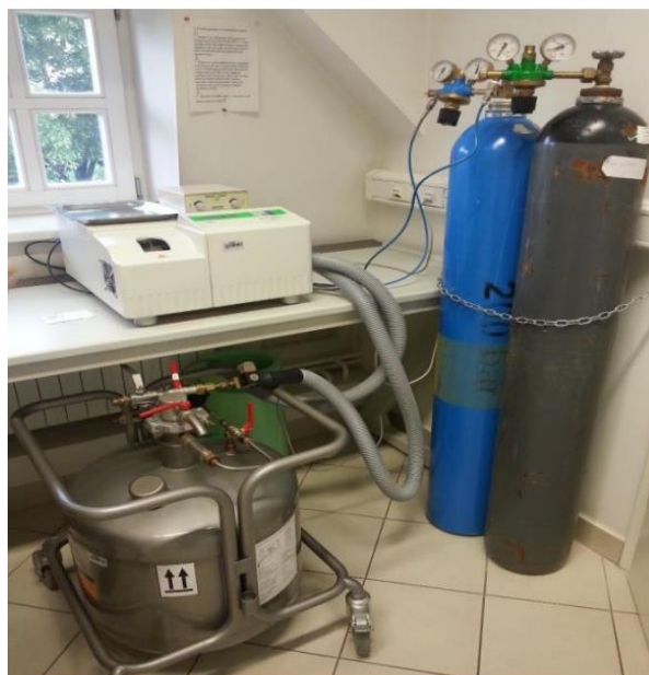
Slika 12. DSC instrument Mettler Toledo DSC 822e
