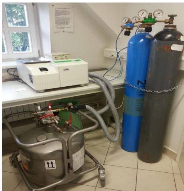
Slika 12. DSC instrument Mettler Toledo DSC 822e
