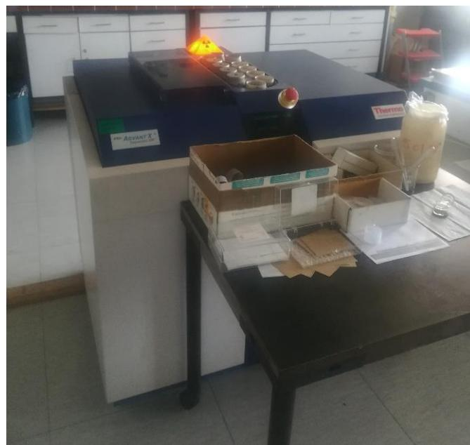
Slika 18. Thermo ARL ADVANT'X+ Sequential XRF
