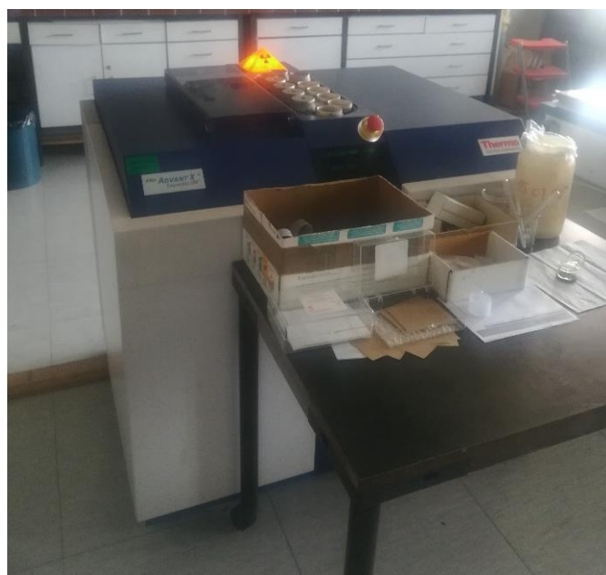
Slika 18. Thermo ARL ADVANT'X+ Sequential XRF
