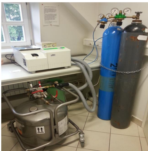
Slika 21. DSC instrument Mettler Toledo DSC 822 e
