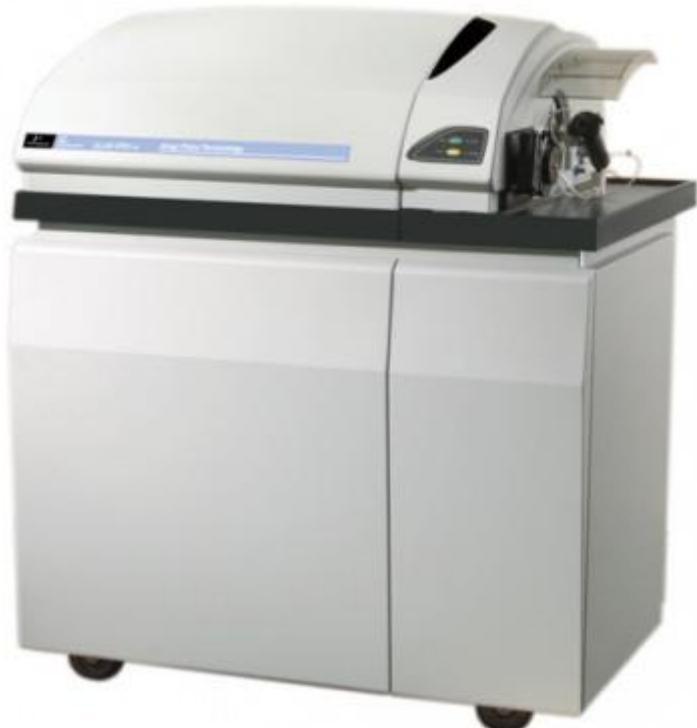
*Slika 13.* ICP-Q-MS uređaj, PerkinElmer ELAN DRC
