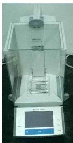
**Slika 3.2.2.** Analitička vaga Mettler Toledo XA105 Dual Range
