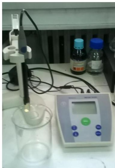
**Slika 3.2.4. pH-metar Mettler Toledo S20 SevenEasy**
