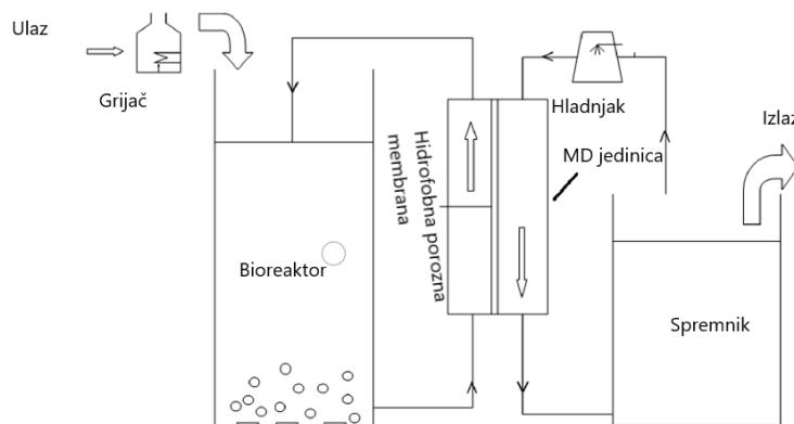
Slika 18. MDBR reactor<sup>24</sup>
