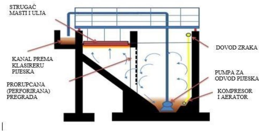
Slika 2. Princip rada mastolova <sup>1</sup>
