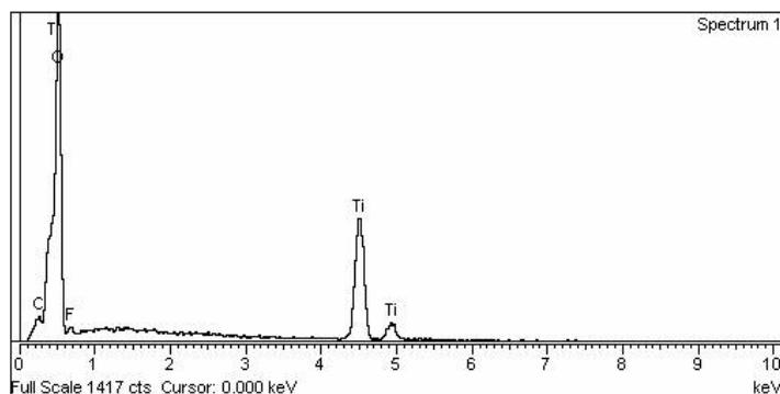
Slika 13. EDXS prikaz  $\text{TiO}_2$  nanocjevčica bez  $\text{BaTiO}_3$
