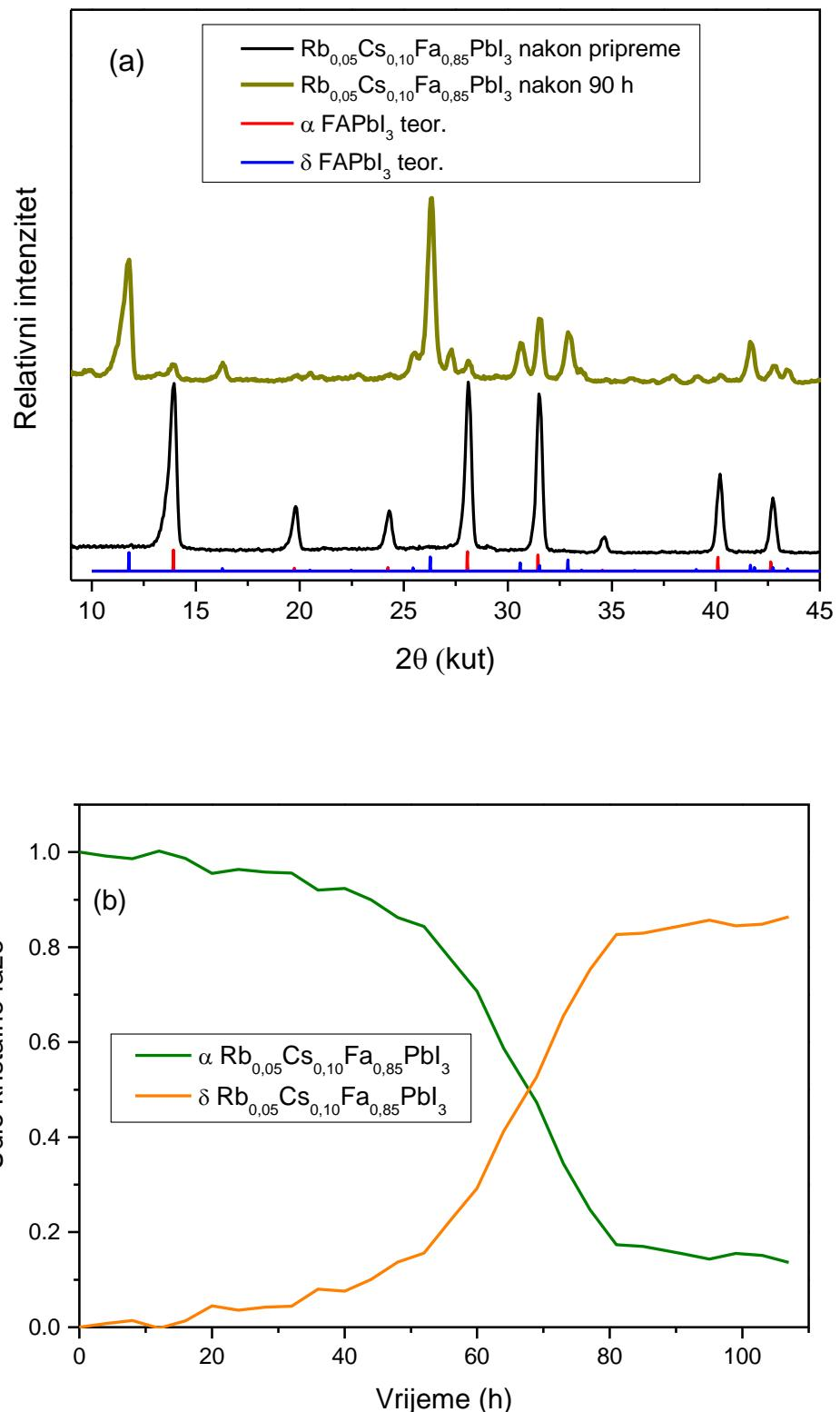
Slika 38. (a) Difraktogram  $\text{Rb}_{0.05}\text{Cs}_{0.10}\text{FA}_{0.85}\text{PbI}_3$  perovskita nakon sinteze i nakon 90 sati; (b) relativni intenziteti [100] ravnine  $\text{Rb}_{0.05}\text{Cs}_{0.10}\text{FA}_{0.85}\text{PbI}_3$  perovskita u vremenu.
