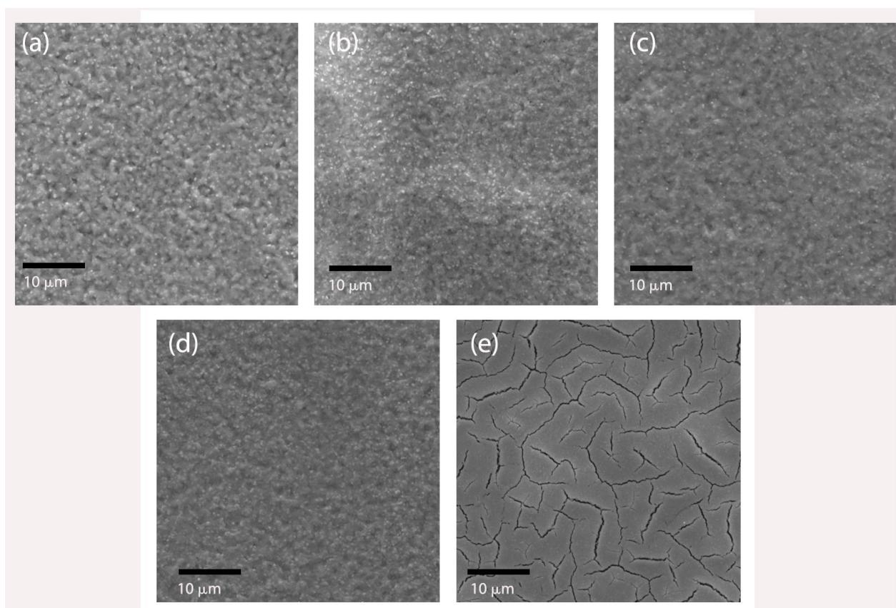
Slika 26. SEM slike  $\text{FAPbI}_3$  tankih filmova u otapalima: (a) čisti DMSO, (b)  $V(\text{DMSO}):V(\text{DMF}) = 4:1$ , (c)  $V(\text{DMSO}):V(\text{DMF}) = 1:1$ , i (d)  $V(\text{DMSO}):V(\text{DMF}) = 1:4$  i (e) čisti DMF.
