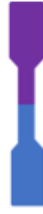
Figure 4.26. Schematic presentation of the tensile test specimen printed one half with visible light and the other half by UV light
