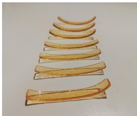
Figure 4.11. Warping of samples of the DOM:ECC = 25:75 system after the thermal treatment
