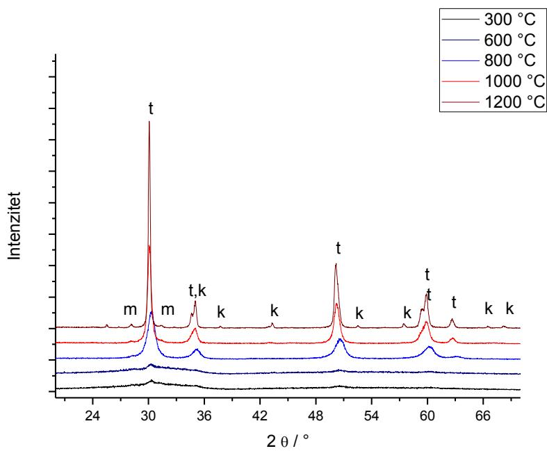
**Slika 14.** Difraktogram uzorka sgA20m; t – t-ZrO<sub>2</sub>, m – m-ZrO<sub>2</sub>, k – korund ( $\alpha$ -Al<sub>2</sub>O<sub>3</sub>)
