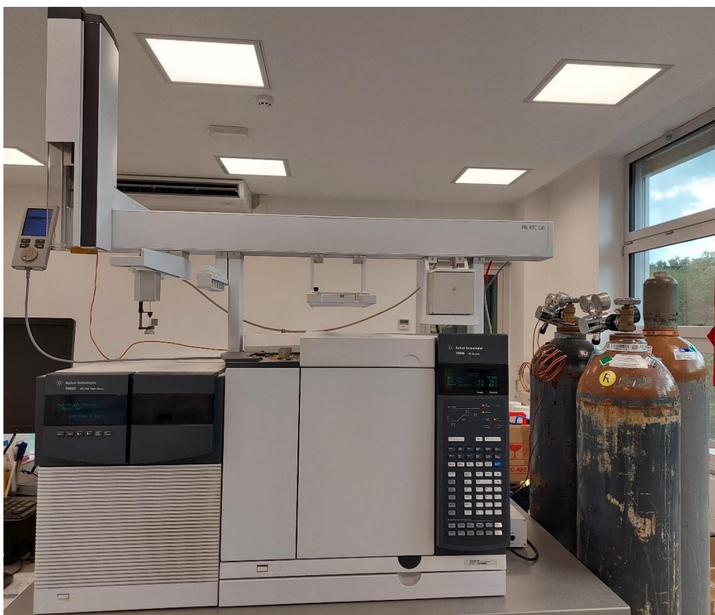
Slika 9. Plinski kromatograf (7890B, Agilent) s trostrukim kvadrupolnim spektrometrom masa (7000C, Agilent)
