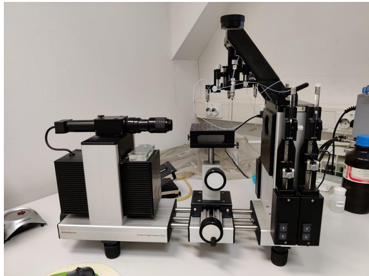
Slika 20. Goniometar DataPhysics OCA 20 Instruments GmbH
