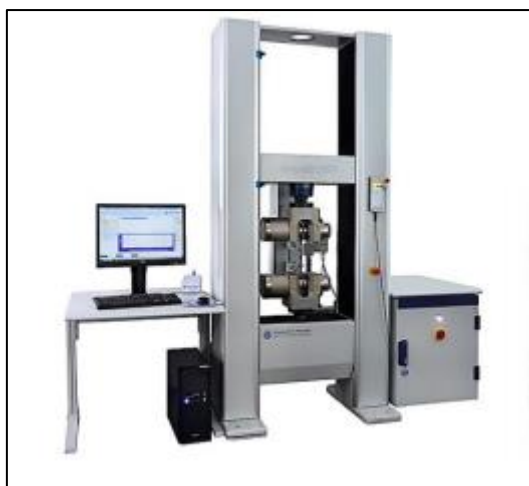
Slika 3.2. Mehanička kidalica ZWICK Testing Machine 1445
