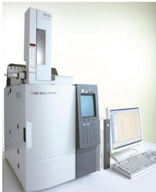
Slika 14. GC – 2014, Shimadzu kolona Carbowax 20M [39]
