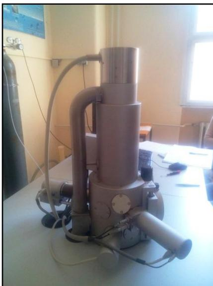
Slika 3.8 SEM Tescan Vega III Easyprobe
