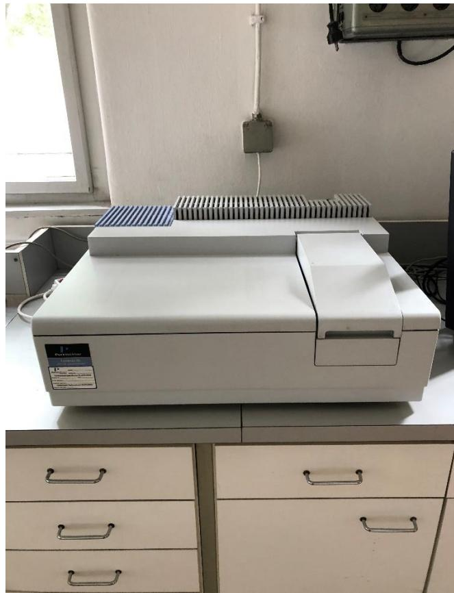
**Slika 7.** Lambda 35 UV/VIS spectrometer, PerkinElmer
