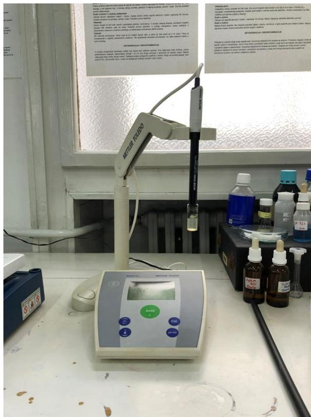
**Slika 6.** pH-metar S20 SevenEasy, Mettler Toledo
