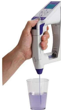
**Slika 10.** Mettler Toledo™ Densito™ 30PX Density Meter [54]
