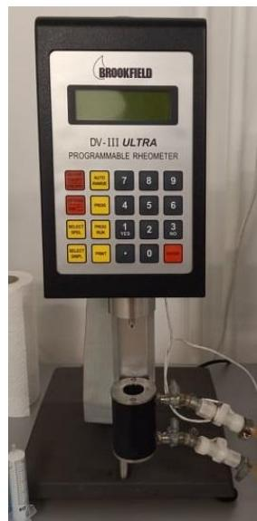
**Slika 11.** Reometar DV-III Ultra Rheometer by AMETEK Brookfield
