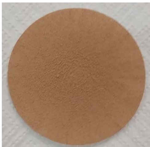
Figure S6. Photo image of immobilized 5% (w/w) \text{Fe}_2\text{O}_3/\text{TiO}_2 nanocomposite onto glass support
