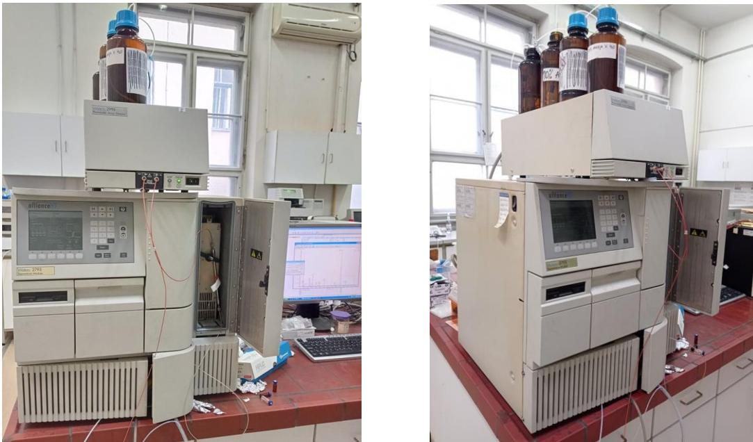
**Slika 24.** Uređaj Waters 2795 Alliance HPLC systems s 2996 PDA detektorom
