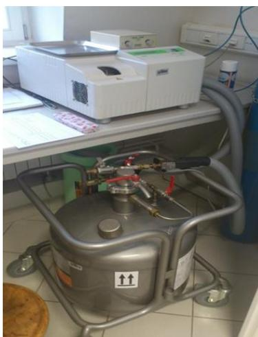
**Slika 10.** DSC instrument Mettler Toledo DSC 822<sup>e</sup>
