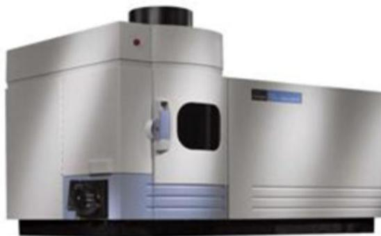
*Slika 18. ICP-OES spektrometar, Perkin Elmer, Optima 2000 DV*
