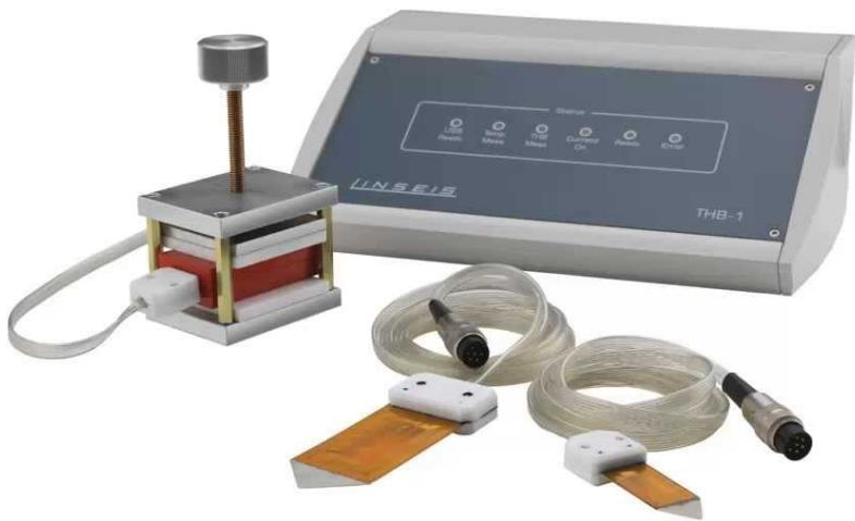
Slika 9. *Transient Hot Bridge (THB) Thermal Conductivity Meter.*
