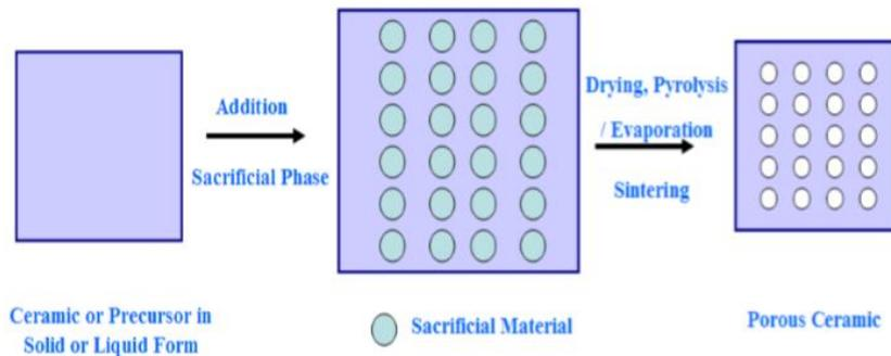
Slika 8.<sup>3</sup> Shematski prikaz sacrificial phase technique
