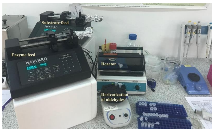
Figure 22 Fed-batch setup for the DERA Tm - and DERA 024 -catalyzed reaction.
