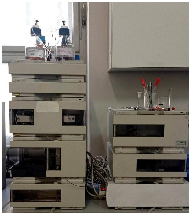
Slika 22. HPLC Agilent Series 1100 s DAD detektorom
