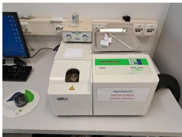
Slika 28. DSC instrument 823<sup>e</sup> Mettler Toledo
