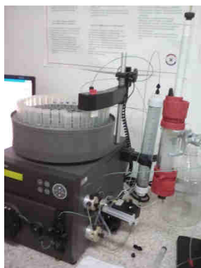
Figure 7.2 Protein purification on Äkta prime plus system.
