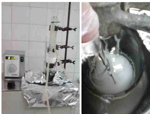
Figure 7.3 Experimental set-up for performing chemical oxidation of 7A .
