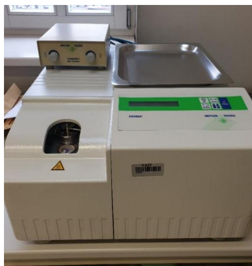
Slika 22. DSC instrument, Mettler Toledo DSC 822 e
