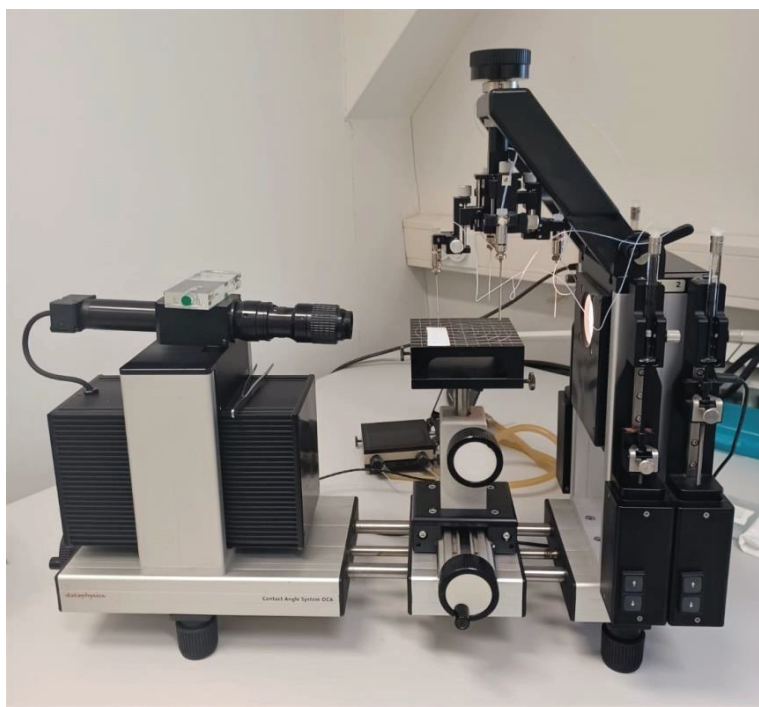
Slika 17. Goniometar DataPhysics OCA 20 Instruments, GmbH
