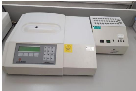
**Slika 3.7.** Luminometar LUMISTox 300 i termometar LUMIStherm, Hach-Lange GmbH.
