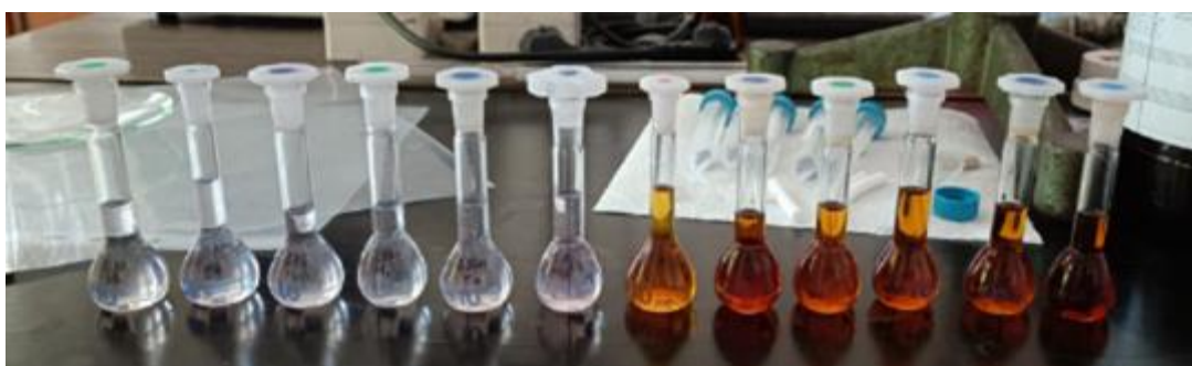
Slika 8. Otopine nitratnih soli ( \text{Mn}(\text{NO}_3)_2 \times 4 \text{H}_2\text{O} i \text{Fe}(\text{NO}_3)_3 \times 9 \text{H}_2\text{O} ) – katalitički prekursori
