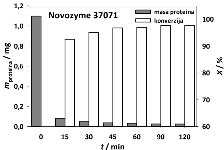
Slika 4.2. Masa proteina i konverzija tijekom hidrolize proteina u ostacima kozica katalizirana proteazama u kotlastom reaktoru ( $T = 50^\circ\text{C}$ ,  $50 \text{ mmol dm}^{-3}$  Tris-HCl pH 8,  $V_{\text{reaktor}} = 200 \mu\text{L}$ ,  $m_{\text{kozica}} = 20 \text{ mg}$ ,  $A_{\text{proteaze}} = 1 \text{ U}$ )
