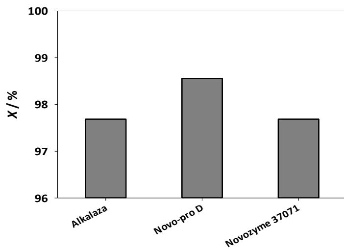
Slika 4.3. Usporedba konverzija tijekom hidrolize proteina u ostacima kozica katalizirana proteazama u kotlastom reaktoru ( $T = 50^\circ\text{C}$ ,  $50 \text{ mmol dm}^{-3}$  Tris-HCl pH 8,  $V_{\text{reaktor}} = 200 \mu\text{L}$ ,  $m_{\text{kozica}} = 20 \text{ mg}$ ,  $A_{\text{proteaze}} = 1 \text{ U}$ )
