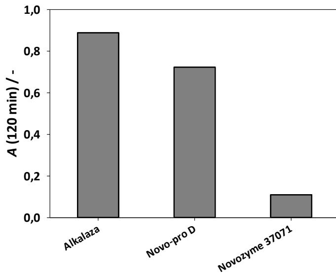
Slika 4.6. Usporedba preostale aktivnosti enzima nakon hidrolize proteina u ostacima kozica katalizirane proteazama u kotlastom reaktoru (  $t = 120 \text{ min}$ ,  $T = 50 \text{ }^{\circ}\text{C}$ ,  $50 \text{ mmol dm}^{-3}$  Tris-HCl pH 8,  $V_{\text{reaktor}} = 200 \mu\text{L}$ ,  $m_{\text{kozica}} = 20 \text{ mg}$ ,  $A_{\text{proteaze}} = 1 \text{ U}$  )
