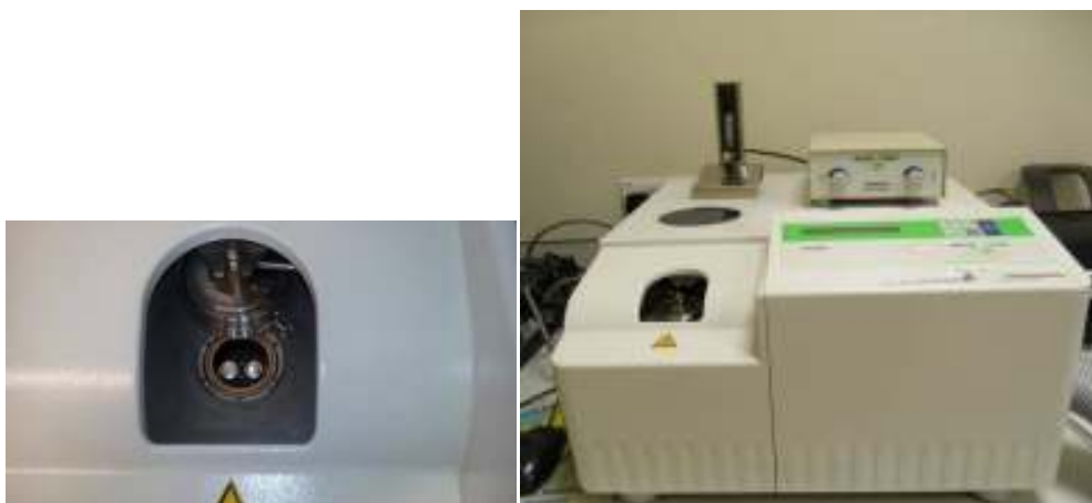
Slika 18. DSC instrument Mettler Toledo DSC 822 e .
