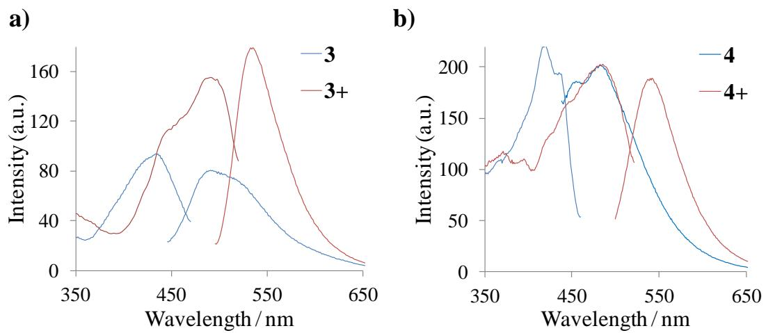
**Fig. S2.** Excitation and emission spectra of compounds **3** and **4**,  $c = 1 \times 10^{-5} \text{ M}$ , in neutral and protonated form in ethanol. (Excitation wavelength at absorption maximum of corresponding species.)
