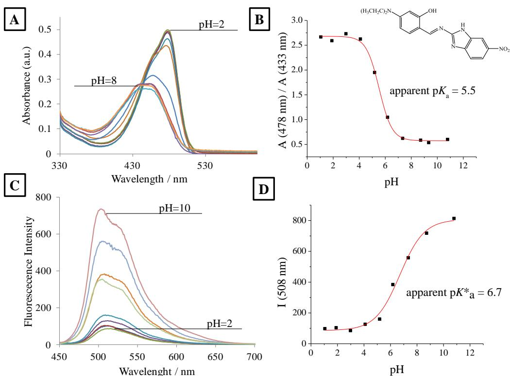
**Figure 5.** Effect of pH on absorption properties of immobilised **3** (A); pH response on selected absorbance wavelength (B); Effect of pH on emission properties of immobilised **3** (C); pH response on selected emission wavelength (D),  $\lambda_{\text{exc}} = 433 \text{ nm}$ .
