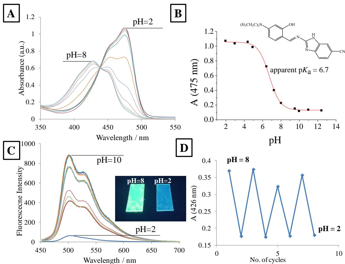
**Figure S6.** Effect of pH on absorbance (a) and emission (b) properties of immobilised **2**; pH response on selected wavelength (b) and results of reversibility of pH response (d),  $\lambda_{exc} = 427$  nm. Inset: photographs of thin films taken under UV lamp.
