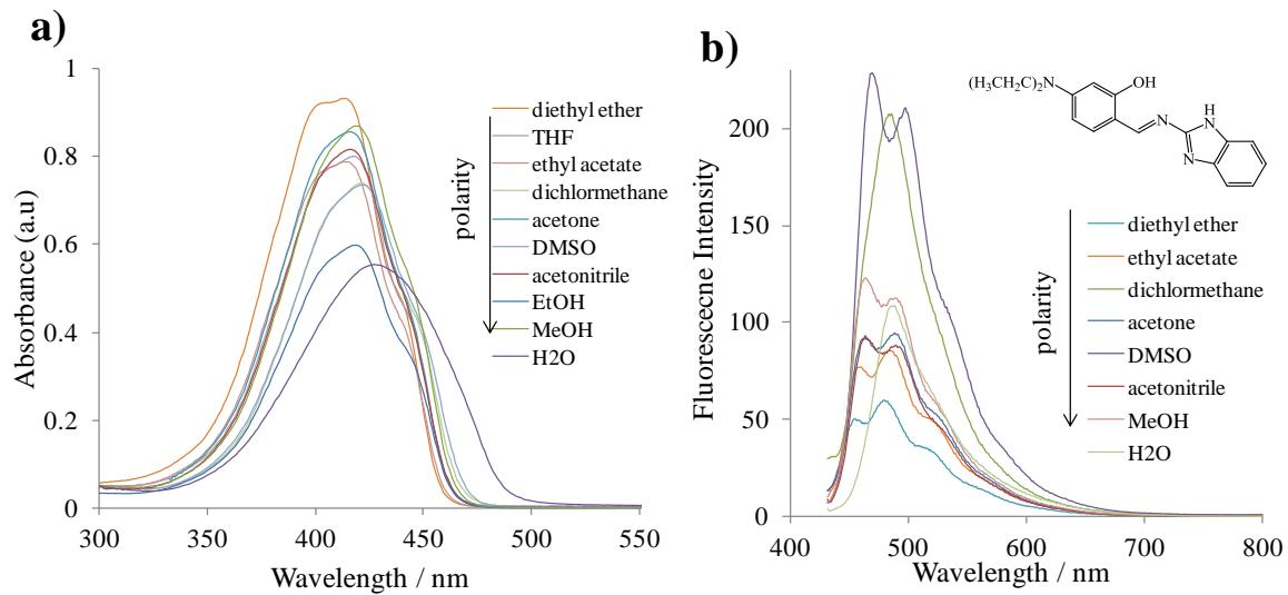
**Figure S1.** UV-vis,  $c = 1 \times 10^{-5}$  M (a) and emission (b) spectra,  $c = 2 \times 10^{-6}$  M of **1** in solvents of different polarity parameter,  $\lambda_{\text{exc}} = \lambda_{\text{abs}}$ .
