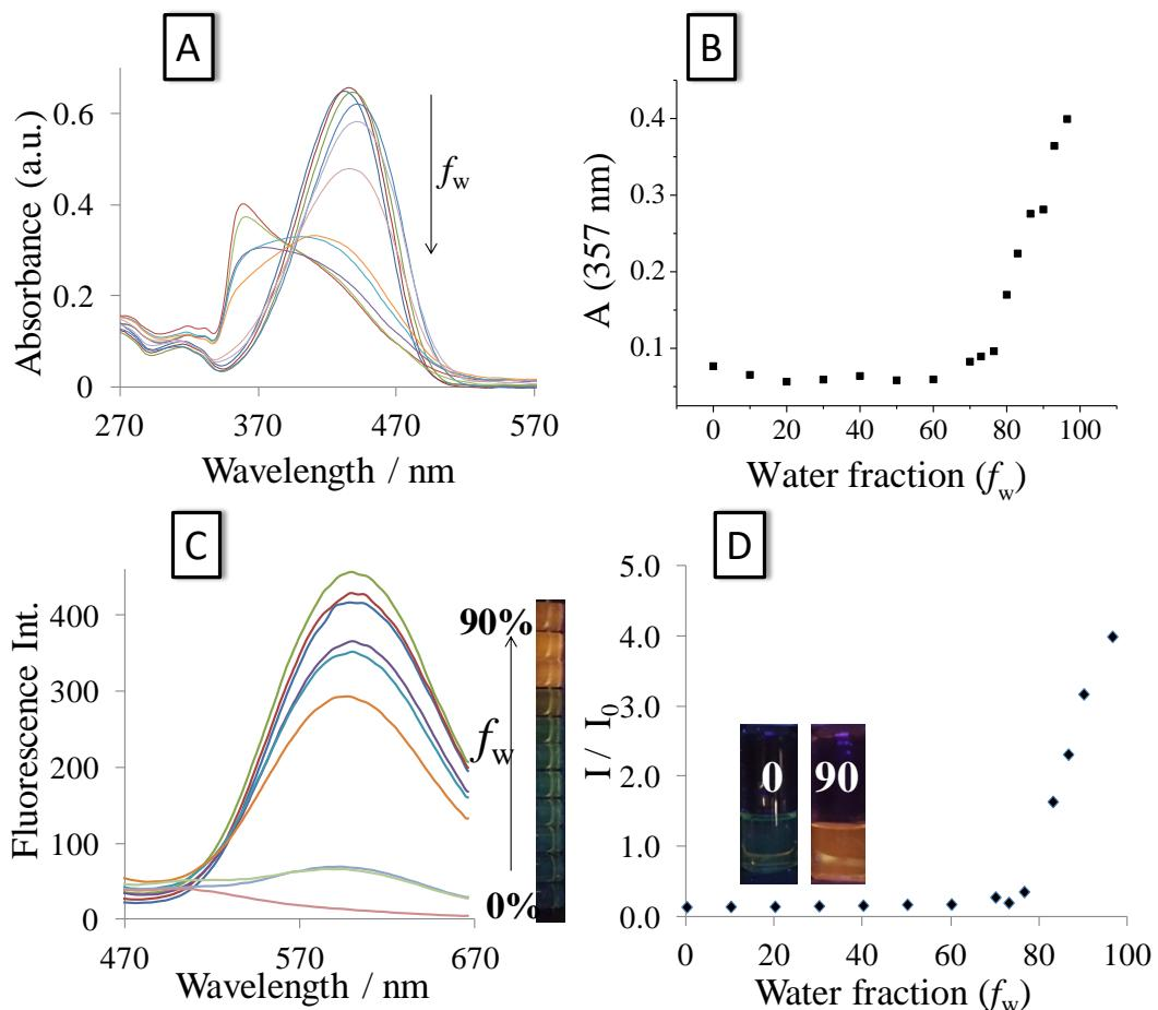
**Figure 3.** (A) Absorption and (C) emission spectra of **BIA** in DMSO at different volume fraction of water; effect of water fraction on the absorption (B) and emission (D) intensity,  $c = 10 \mu\text{M}$ ,  $\lambda_{\text{exc}} = 350 \text{ nm}$ .
