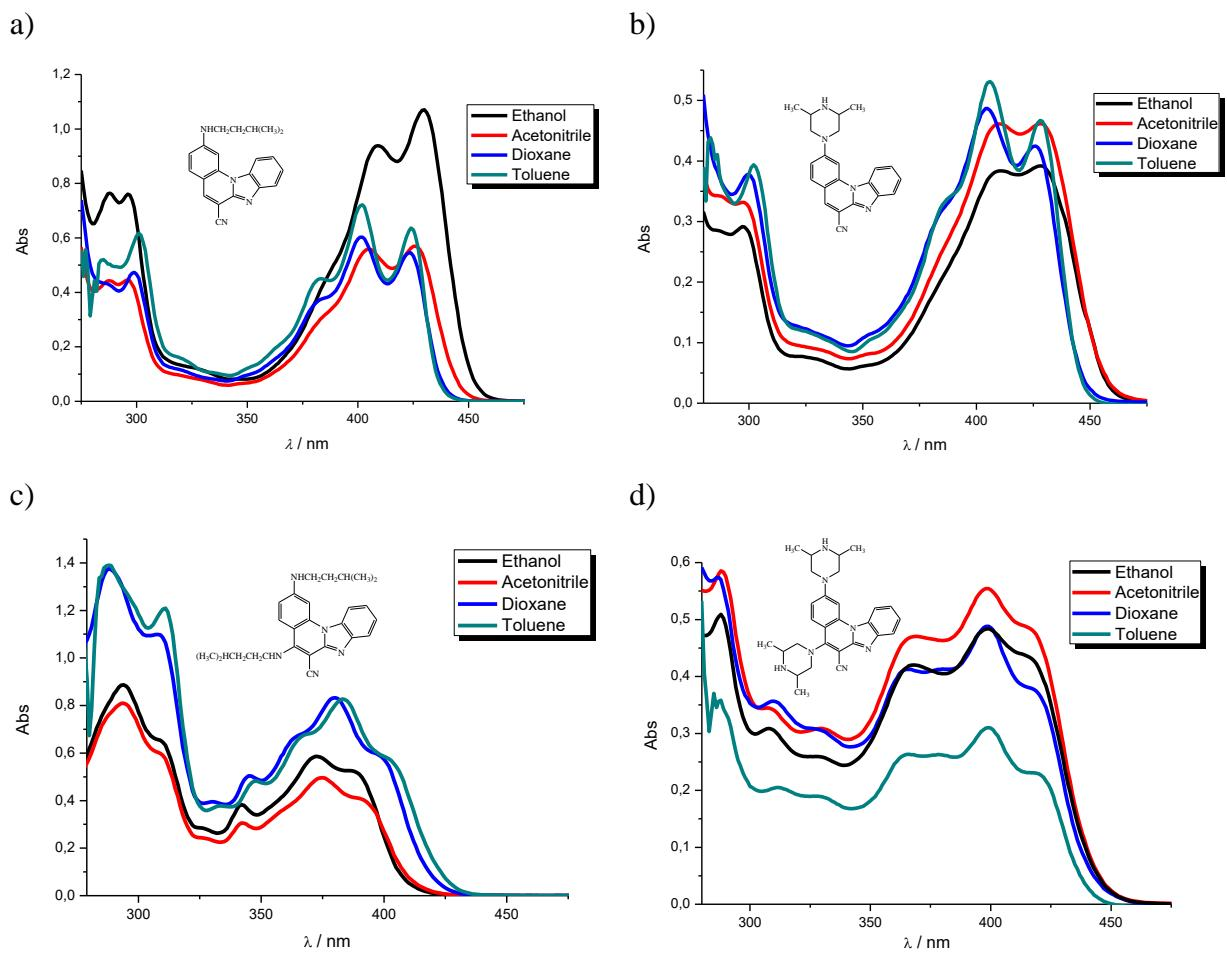
Figure 1. UV-Vis spectra recorded in ethanol, acetonitrile, dioxane and toluene at concentration of  $2 \times 10^{-5}$  mol dm $^{-3}$  of 3 (a), 4 (b), 5 (c) and 6 (d).
