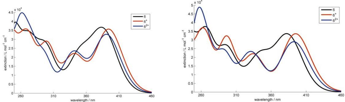
**Figure S5.** TD-DFT calculated UV/Vis spectra of **6** and its monoprotonated (**6<sup>+</sup>**) and diprotonated (**6<sup>2+</sup>**) derivatives in water obtained at the (IEF-PCM)/M06/6-311++G(2d,2p) (top) and (IEF-PCM)/M06/6-31+G(d) (bottom) levels of theory.
