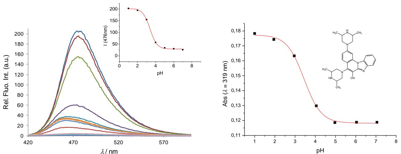
**Figure 4.** Fluorescence emission spectra of **6**,  $2 \times 10^{-6}$  mol dm $^{-3}$  at different pH values (left) and its calibration curve (right); absorbance versus pH at 319 nm.
