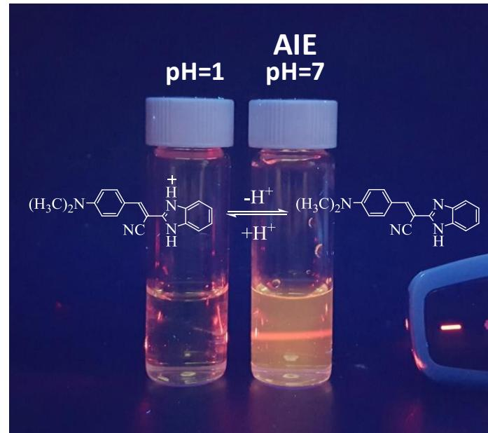
**Fig. S10.** Observation of the Tyndall effect on nanoaggregates; a red laser beam is directed through solutions of **BIA** in water at pH = 7 (right) and at pH = 1 (left). Nanoaggregates of **BIA** in the water cause light scattering, seen as a *red-line* through the solution. Light scattering at pH = 1 is not observed.
