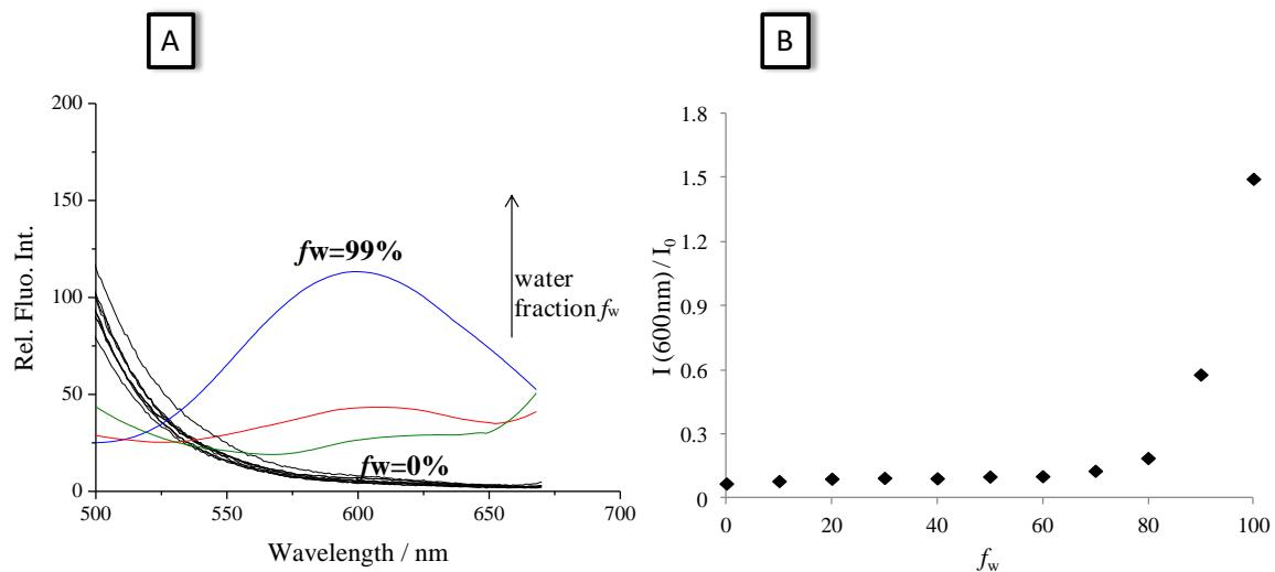
**Fig. S3.** (A) Emission spectra of **BIA** in THF at different volume fraction of water; (B) Effect of water fraction on emission intensity,  $c = 10\mu\text{M}$ ,  $\lambda_{\text{exc}}=350\text{ nm}$ .
