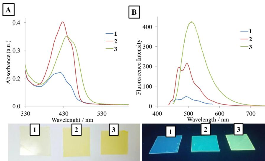
**Figure 3.** UV-vis absorption (a) and emission (b) spectra of chemosensors **1-3** in plasticised PVC thin films; photographs taken in daylight and under UV lamp ( $\lambda_{\text{exc}} = 366 \text{ nm}$ ).
