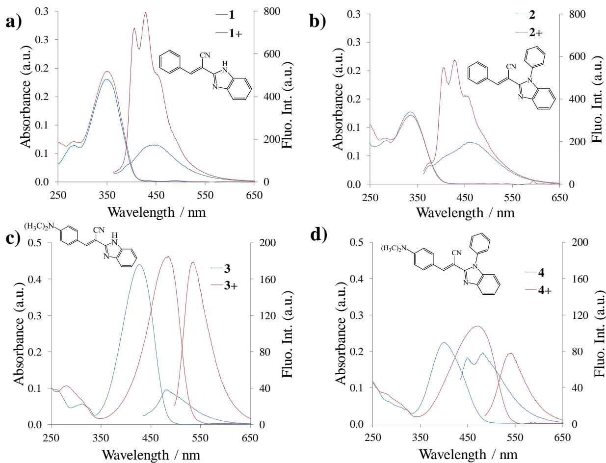
**Fig. 6.** Absorption and emission spectra of compounds **1**–**4**,  $c = 1 \times 10^{-5}$  M, in neutral and protonated form in ethanol. (Excitation wavelength at absorption maximum of corresponding species.)
