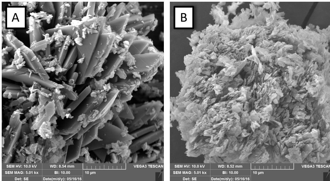
**Fig. S6.** SEM images of aggregates prepared by precipitation method in (A) **THF/water** and (B) **ethanol/water** mixtures. The former exhibits an irregular distribution of crystal sizes, where the larger crystals are of regular rhomboidal shape and tend to aggregate. The latter has a more uniform size distribution, with nanoparticles self-assembled in aggregates of dimension  $\sim 250$  nm.
