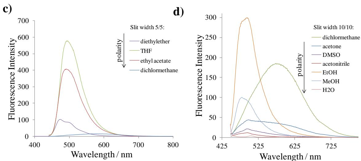
**Figure S2.** UV-vis,  $c = 1 \times 10^{-5}$  M (a) and emission (c,d) spectra,  $c = 2 \times 10^{-6}$  M of **3** in solvents of different polarity parameter,  $\lambda_{\text{exc}} = \lambda_{\text{abs}}$ ; photographs of **3** in solvents of increasing polarity taken on day light and under UV lamp (b).
