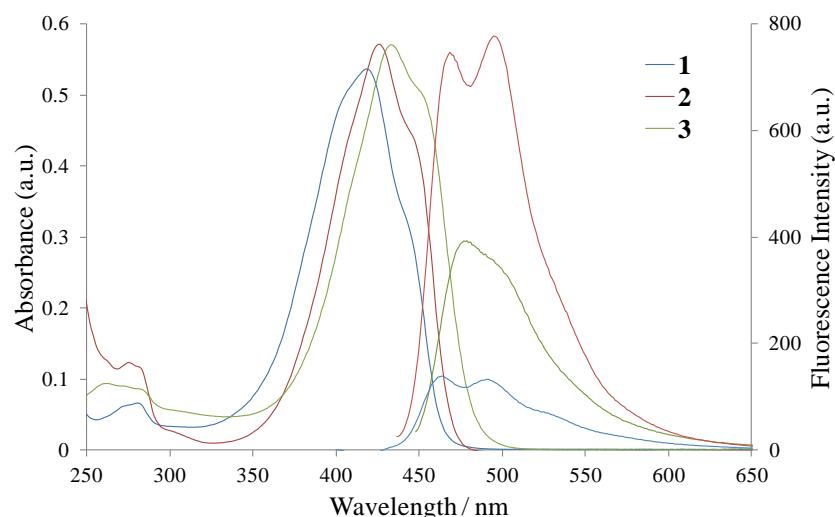
**Figure 1.** UV-vis absorption and emission spectra of chemosensors **1-3** in ethanol.
