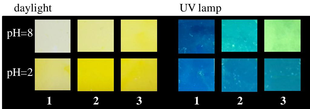
**Figure 6.** Photographs of thin polymer films of **1-3** taken in daylight and under UV lamp ( $\lambda_{\text{exc}} = 366 \text{ nm}$ ) showing the changes upon protonation
