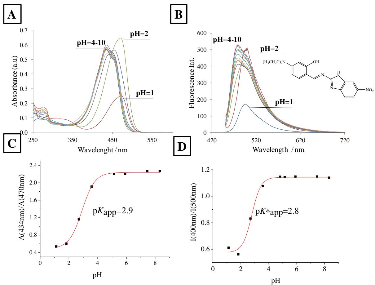
**Figure S4.** Effect of pH on absorbance (A) and emission (B) properties of **3**; pH response at chosen absorbance wavelength (A) and emission wavelength (D); ( $c = 10 \mu\text{M}$  and  $2 \mu\text{M}$ ,  $\lambda_{\text{exc}} = 433 \text{ nm}$ ).
