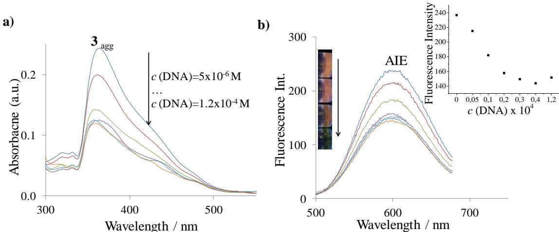
**Fig. 10.** a) Absorption and b) emission spectra ( $\lambda_{\text{exc}} = 350 \text{ nm}$ ) of **3** in aqueous solution (buffer pH = 7.0) upon titration with DNA.
