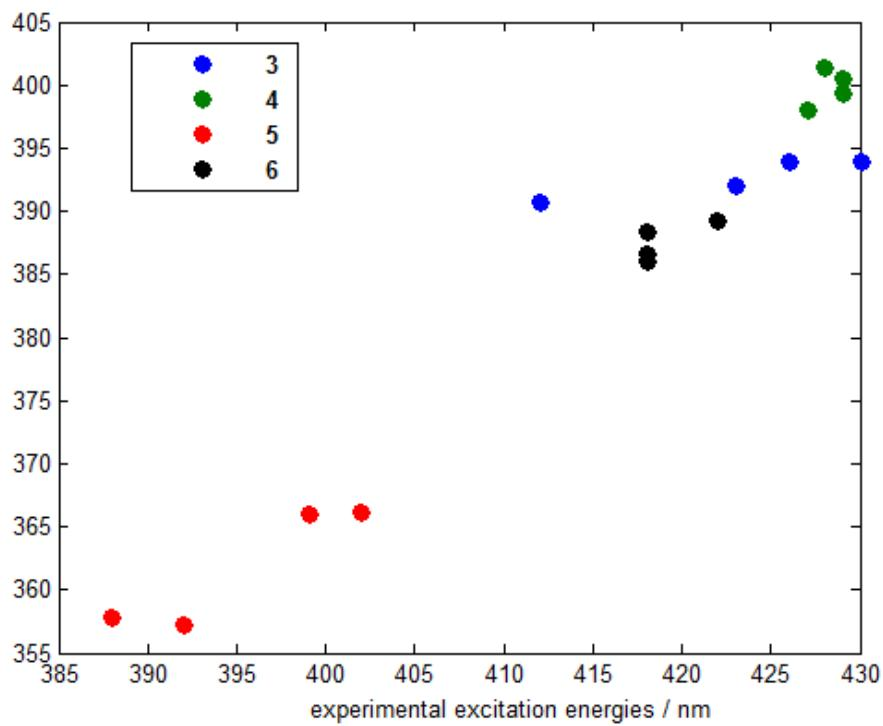
**Figure S8.** Correlation between the calculated and experimental lowest excitations for systems **3–6** in different solvents. Only the first excitation energies are shown (the solvents are not labeled). Linear regression reveals a reasonable correlation ( $\lambda_{\text{CALC}} = 1.058 \cdot \lambda_{\text{EXP}} - 55.07$ ) with the regression coefficient of  $R^2 = 0.94$ .
