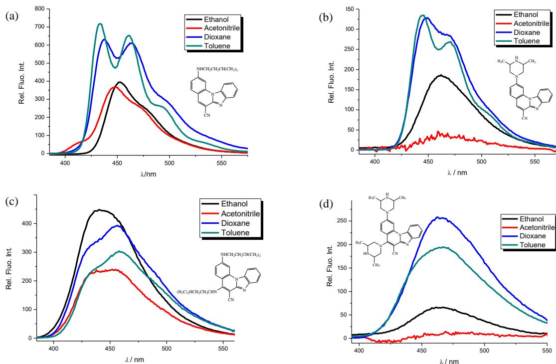
**Figure 2.** Fluorescence emission spectra in ethanol, acetonitrile, dioxane and toluene at concentration of  $1 \times 10^{-7}$  mol dm $^{-3}$  of **3** (a), **4** (b), **5** (c) and **6** (d),  $\square_{\text{exc.}} = 300\text{nm}$ .
