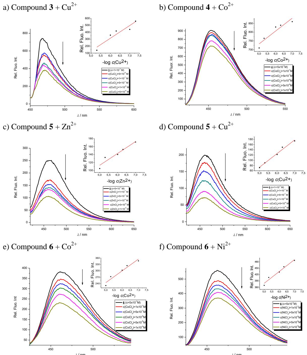
**Figure 6.** Fluorimetric titrations of compound **3** with Zn<sup>2+</sup> (a), **4** with Co<sup>2+</sup> (b), **5** with Zn<sup>2+</sup> (c) and Cu<sup>2+</sup> (d) and **6** with Co<sup>2+</sup> (e) and Ni<sup>2+</sup> cations (f).
