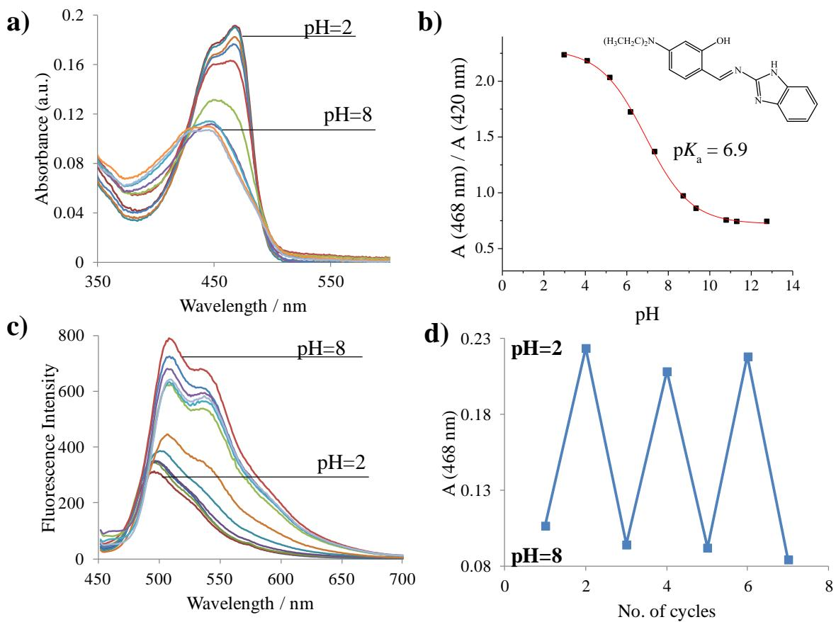
**Figure S5.** Effect of pH on absorbance (a) and emission (b) properties of immobilised **1**; pH response on selected wavelength (b) and results of reversibility of pH response (d),  $\lambda_{\text{exc}} = 417$  nm.
