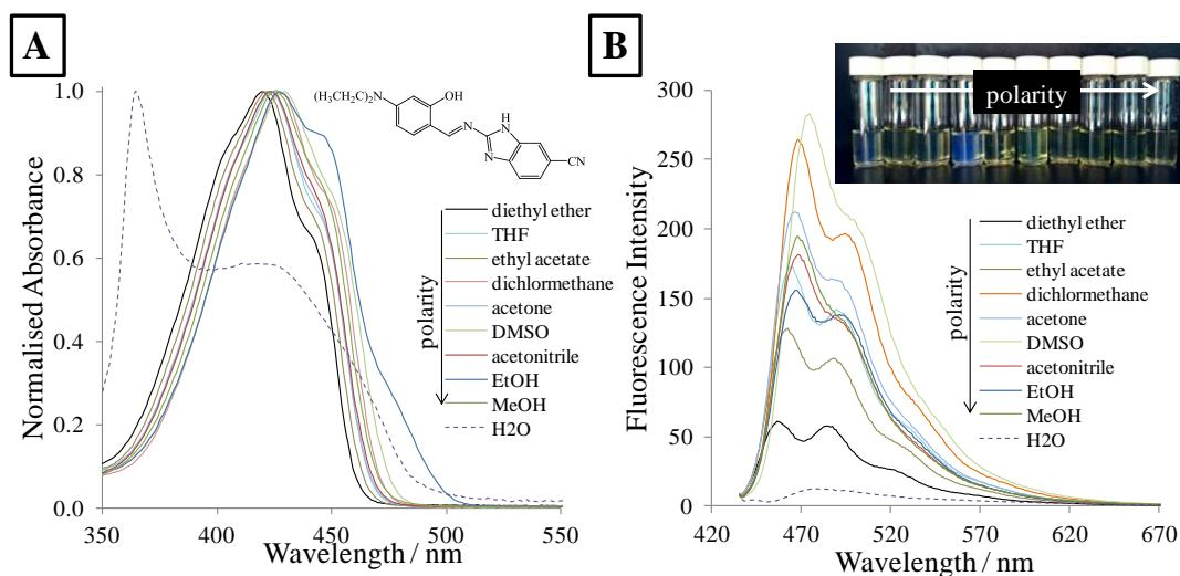
**Figure 2.** UV-vis,  $c = 1 \times 10^{-5}$  M (a) and emission (b) spectra,  $c = 2 \times 10^{-6}$  M, of **2** in solvents of different polarity parameter,  $\lambda_{\text{exc}} = \lambda_{\text{abs}}$ .
