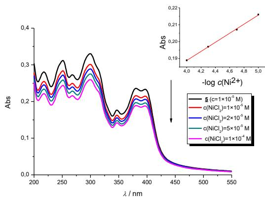
**Figure 5.** UV-Vis titrations of compound **3** with Zn<sup>2+</sup> (a) and Cu<sup>2+</sup> cations (b) and titrations of compound **5** with Zn<sup>2+</sup> (c) and Ni<sup>2+</sup> cations (d).
