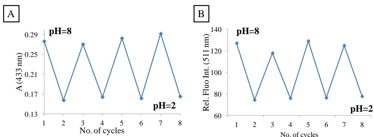
**Figure 7.** Reversible pH response of **3** (protonated – neutral) at selected absorbance ( $\lambda = 433$  nm) and emission wavelength  $\lambda = 511$  nm),  $\lambda_{\text{exc}} = 433$  nm.
