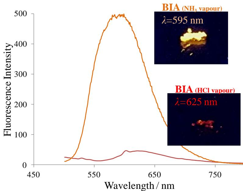
**Figure 7.** Emission spectra of **BIA** in solid state and upon exposure to the vapours of HCl ( $\mathbf{BIA}^+$ ),  $\lambda_{\text{exc}}=440 \text{ nm}$ .
