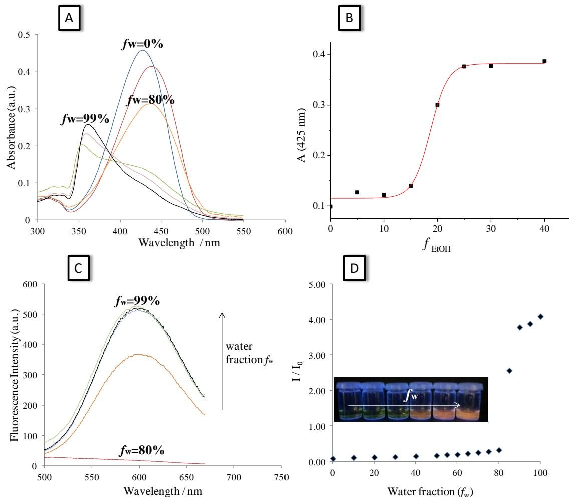
**Fig. S2.** (A) Absorption and (C) emission spectra of **BIA** in **ethanol** at different volume fraction of water; effect of water fraction on (B) absorbance and (D) emission intensity,  $c = 10 \mu\text{M}$ ,  $\lambda_{\text{exc}} = 350 \text{ nm}$ .
