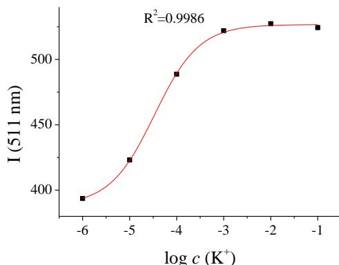
**Figure 8.** Response of the potassium-sensing thin films to different KCl concentrations. The Boltzmann function fit is used for calibration. KCl concentrations range from  $10^{-6}$  M to  $10^{-1}$  M.
