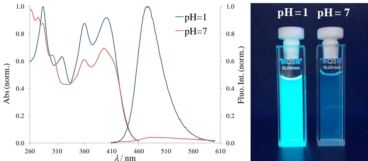
**Figure 3.** Typical absorption and fluorescence emission spectra of compound **6** ( $\lambda_{\text{exc.}}=397$  nm) in buffer at pH = 7 and pH = 1 (bottom).
