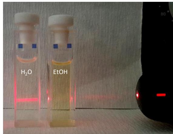
**Fig. S4.** Observation of the Tyndall effect on nanoaggregates; a red laser beam is directed through solutions of **BIA** in water (left) and ethanol (right). Nanoaggregates of **BIA** in the water cause light scattering, seen as a *red-line* through the solution. Light scattering in ethanol solution is not observed.
