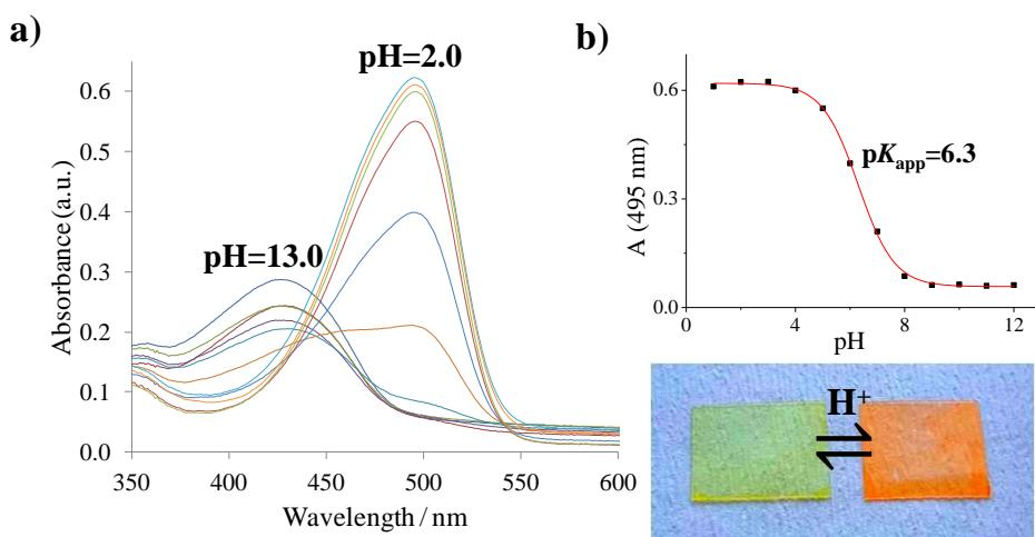
**Fig. 9.** a) Absorbance spectra of chromophore **3** immobilised in plasticised PVC film at different pH values; b) calibration plot of immobilised chromophore **3** (absorbance change in response to pH at 495 nm).
