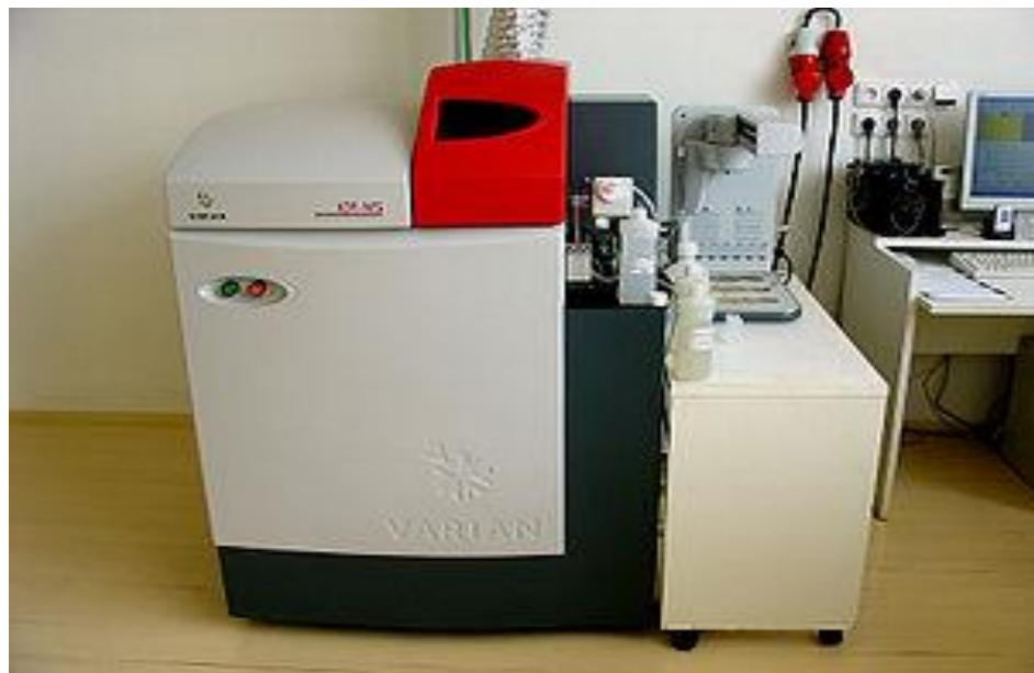
**Slika 32 :** Spektrometar ICP-MS
