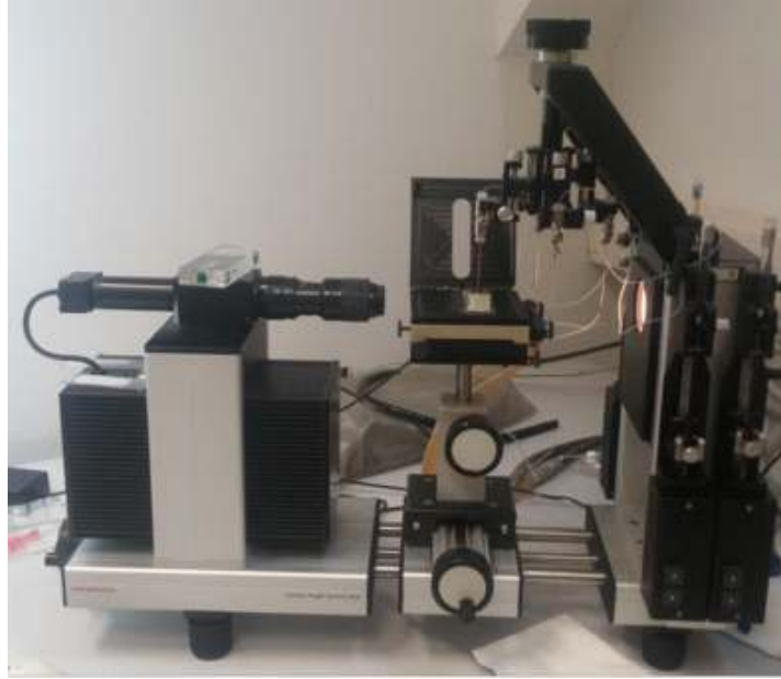
Figure 69: Goniometer DataPhysics OCA 20 for measuring the contact angle
