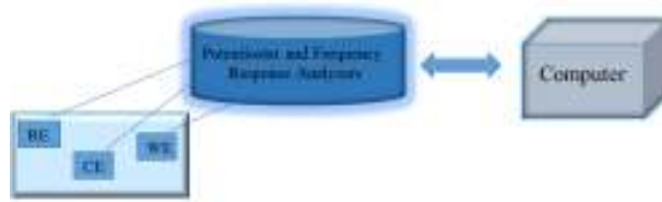
Figure 36: Scheme of electrochemical impedance spectroscopy (EIS) measurements
