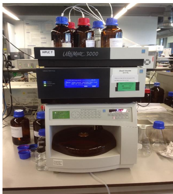
Figure 6 Dionex pump and autosampler
