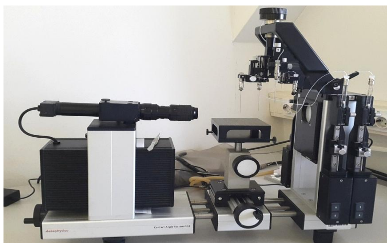
Slika33. Goniometar DataPhysics OCA 20 Instruments, GmbH
