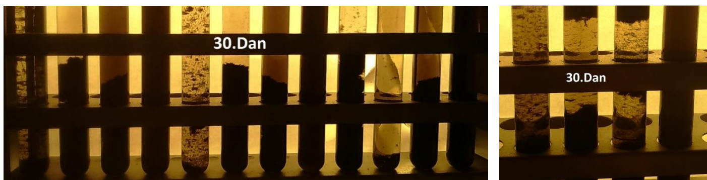
Slika 4.2.14. Sedimentacijski test nanofluida (s lijeva na desno: PDPA, PDPA2, PDPA5, PDPA10, PDPS, PDPS2, PDPS5, PDPS10, YDPA, YDPA2, YDPA5, YDPA10, YDPS, YDPS2, YDPS5, YDPS10), 30. dan
