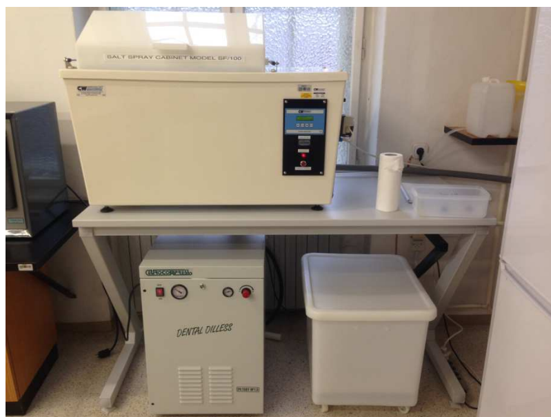
Slika 4. Slana komora (CW specialist equipment model SF/100)
