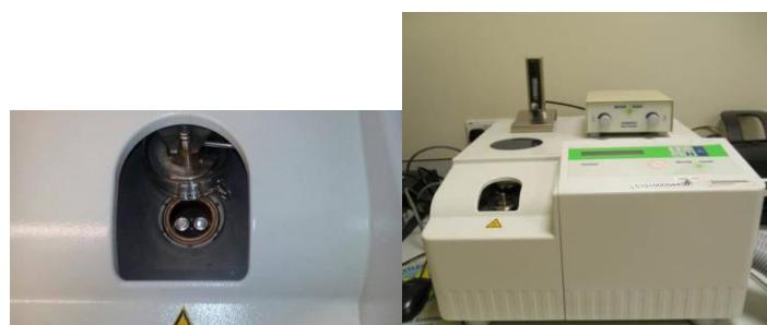
**Slika 13.** DSC instrument Mettler Toledo DSC 822<sup>e</sup>
