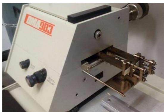
**Slika 14.** DMA 983 TA instruments
