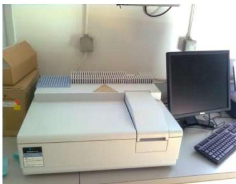
**Slika 3. 1.** UV/VIS spektrofotometarLambda 35 (PerkinElmer, Waltham, SAD)
