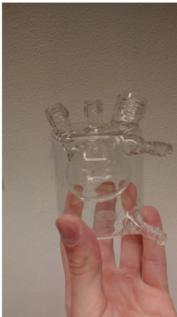
Figure 12. Glass beaker with a jacket that was employed for CV measurements
