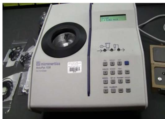
Slika 13. Micromeritics Accupyc 1330
