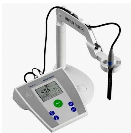
**Slika 8.** pH metar Mettler Toledo, Seven Easy, Švicarska [66]
