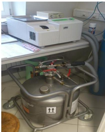
**Slika 11.** DSC instrument Mettler Toledo DSC 822°
